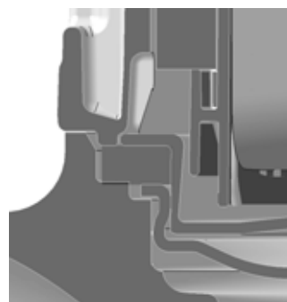
Fig. 37 Sectional drawing showing sealing principle of gasket
