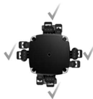
Control box position
