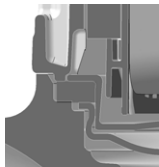
Fig. 37 Sectional drawing showing sealing principle of gasket
