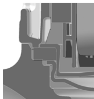
Fig. 37 Sectional drawing showing sealing principle of gasket
