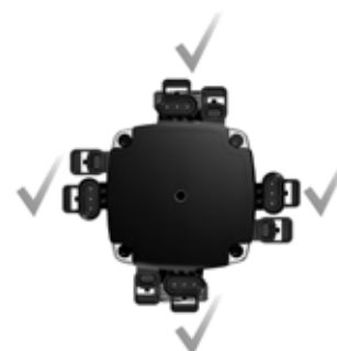
Control box position
