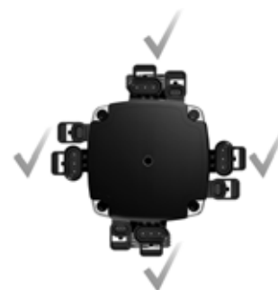
Control box position
